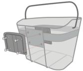
6. Slide the basket down over the bracket until the release tab clicks. Check that the tab is locked by trying to pull up on the basket. It should not move.
