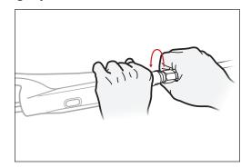
**6.** Use the slide hammer action to remove the bushing.
