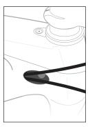
**3.** At the head tube, route the wire through the cable.
