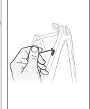
**Technician Tip:** Use a hook tool to help the cable through the chainstay hole.
