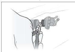
11. Put a new spacer in place around the damper shaft.
