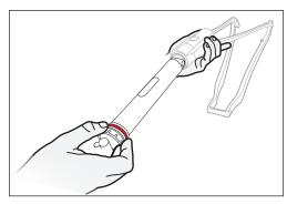
**4.** Push the strut into the carriage until the damper body eyelet is centred with the carriage mount hole.
