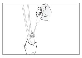
**13.** Firmly press the oil plug back into the aft end of the IsoStrut. Make sure the plug is tightly seated in the IsoStrut opening.
