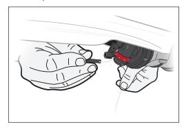
**6.** Route the wire around the lockout spool and install the set screw.
