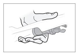
**18.** Use the torque wrench and the hole in the BB wrench to torque the lock ring to 17 Nm.
