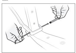
8. From the drive side, insert the other main pivot bolt washer between the front triangle frame and the drive side swing arm. Push the Allen key through the washer.
