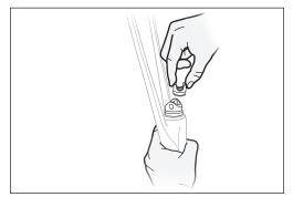
**14.** Install the compression sleeve into the strut cap.
