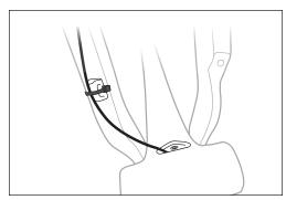
**5.** Route the hose up the down tube and out the left side head tube hole.
