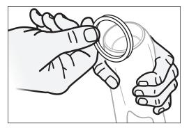
**3.** Use the Delrin rod to pull out the rear seal.
