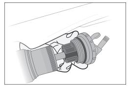
**12.** Depending on the size of the spacer, use the spanner pliers or a parallel jaws pliers to fit the spacer into place.
