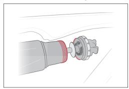
**10.** Move the round metal plate backwards into the IsoStrut. Then use a spanner pliers to remove the air volume spacer.
