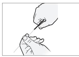
**4.** At the IsoStrut, slide the ferrule on the wire.
