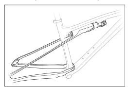
**3.** Install BUT DO NOT TORQUE the aft IsoStrut axle and end cap bolt.
