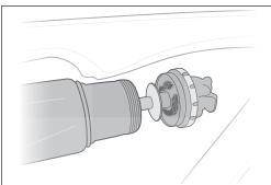
**9.** Clean off any dirt or adhesive residue from the shock threads and the lock ring.
