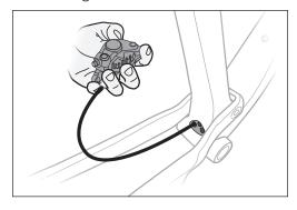
2. Install the rear brake on the chainstay.
