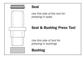
**10.** Put both tools with bushings in the front and rear of the carriage.
