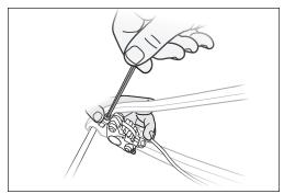
**3.** Route the rear brake hose through the two chainstay cable guides.
