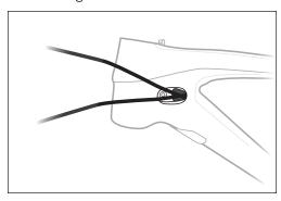
2. Continue to route the cable from the rear cable hole through the rear chainstay hole (drive side).
