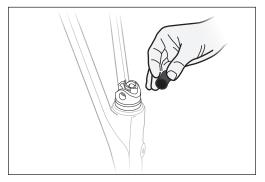
**15.** Wipe off excess oil from assembly when you have finished.
