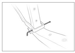
**Technician Tip:** Use the long arm Allen key or similar to properly align the washers on each side of the main pivot joint.
