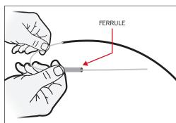
**5.** Guide the wire through the slot in the cable stop.
