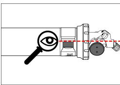
Make sure the air spring valve has enough clearance to the frame to clear your shock pump.
