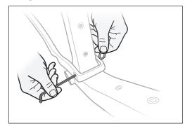
7. Slide the main pivot bolt onto the non-drive side end of the Allen key, through the washer and into the pivot bearing. This will hold the washer and bolt in place. Pull the Allen key out.
