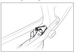
2. Install the centre cable guide plate. Torque the bolts to 2 Nm.
