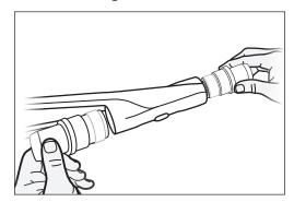
Insert the headset press from the front of the carriage (handle end on the front of carriage).
