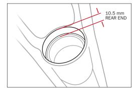
**15.** From the front of the carriage, use the bushing sizer to size the bushing.
