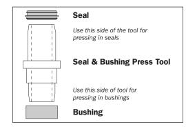
**3.** Put both tools with seals in the front and rear of the carriage.
