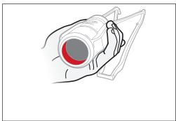
**3.** With the sag o-ring on the strut, insert the IsoStrut into the swing arm carriage.
