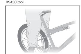
**CAUTION:** Take special care to protect the top tube from scratches that may result from the open-ended tool breaking the lock ring loose.
