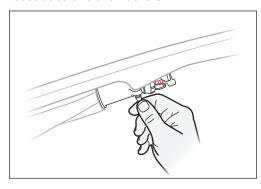
**5.** From the drive side, insert the Allen wrench into the main pivot bearing.
