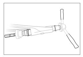
**6.** Spin the headset press down snug. Check for correct alignment of press, tools and seals. Rotate the press to push the seals into place.
