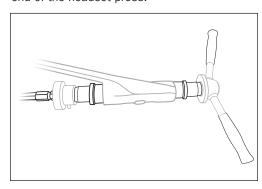
**13.** Spin the headset press down snug. Check for the correct alignment of press, tools and bushings. Rotate the press to push the bushings into place.
