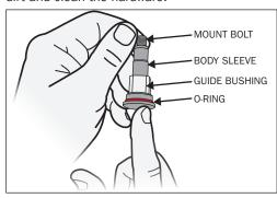
**6.** Inspect the o-ring in the captive nut for wear and excess dirt. Clean or replace as necessary.
