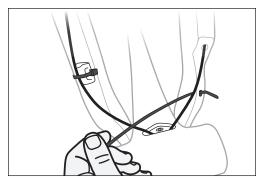
**4.** Connect the rear derailleur to the chainstay. Torque to original manufacturer's specification.
