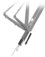
Battery and controller assembly
