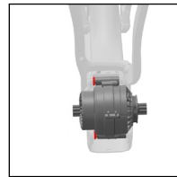
Adjust the compensation screws
