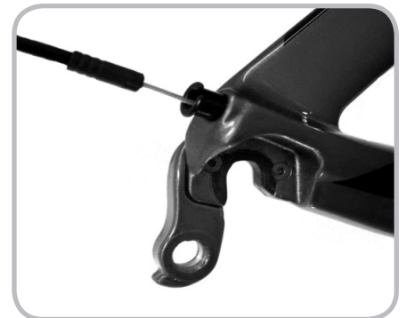
Figure 9.5. Rear derailleur cable passing through the dropout housing stop
