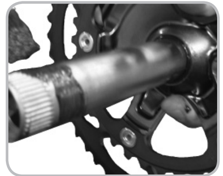
Figure 14.20. Greasing the axle
