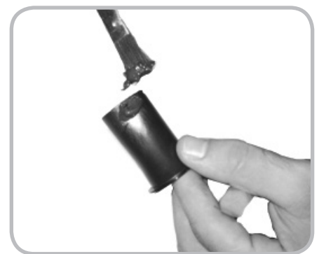
Figure 14.1. Applying grease to the axle shield
