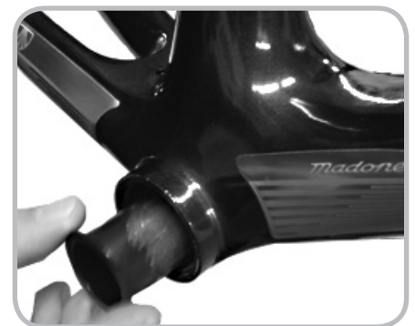
Figure 14.2. Inserting one half of the axle shield into frame
