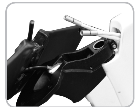
Figure 7.18. Installing the aerobar, ferrule in long position
