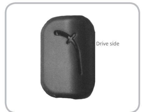
Figure 9.3. Correct orientation of seat tube grommet
