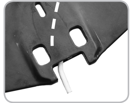
Figure 7.12. Rear brake housing routed out of aerobar (top view of aerobar)
