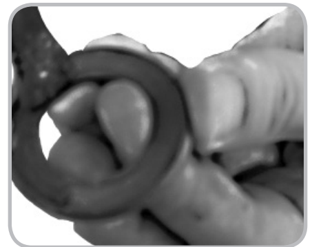
Figure 14.18. Greasing the bearing covers
