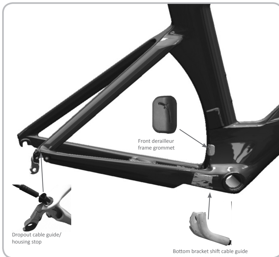
Figure 9.1. Speed Concept parts for shift cable routing
