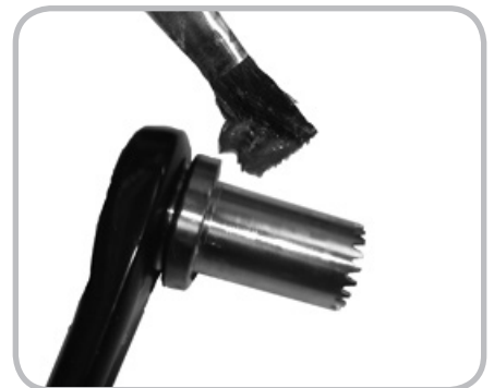
Figure 14.28. Greasing the bearings
