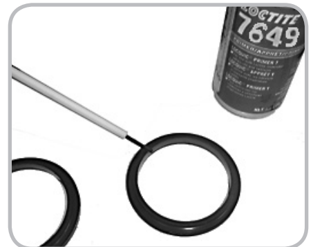
Figure 14.26. Applying Loctite primer to the outer step of the bearing cups
