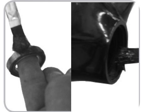
Figure 14.34. Greasing the bearing and the frame saddle
