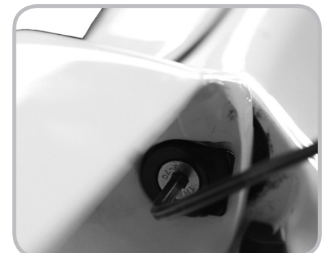
Figure 6.5. Steering lock bolt passes through lock washer and into steering axle
