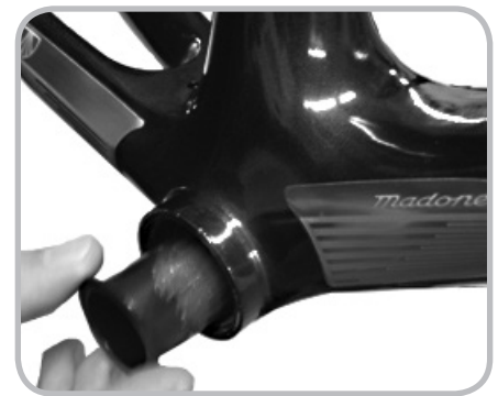
Figure 14.41. Inserting one half of the axle shield into frame
