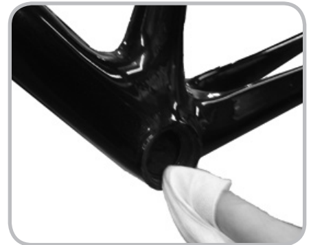
Figure 14.25. Cleaning bonding surfaces with an alcohol wipe
