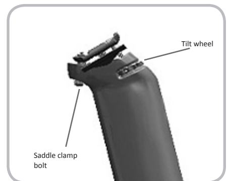
Figure 4.3. Tilt wheel and saddle clamp bolt of saddle angle adjustment mechanism
