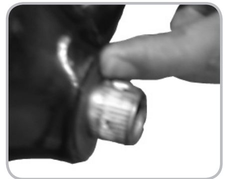
Figure 14.22. Pressing in the second bearing cover
