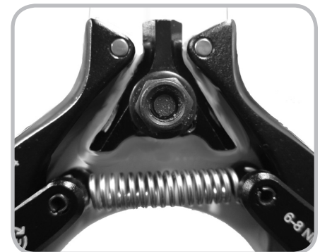
Figure 6.9. Squeeze the lower arms to remove the wedge
