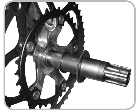
Figure 14.11. Sliding the wave washer and bearing cover onto the axle
