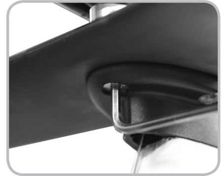
Figure 7.19. Tightening front attachment bolt
