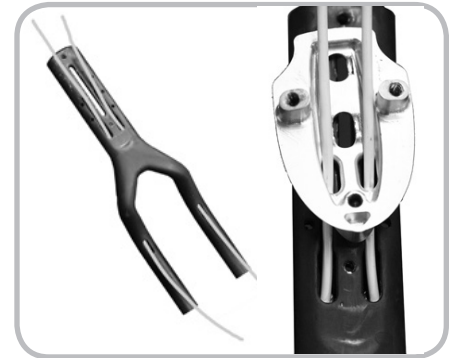
Figure 7.8. Shift housing routed through mono-extension and mono-spacer
