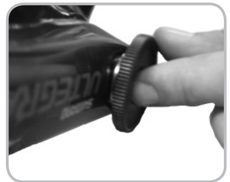
Figure 14.23. Pressing the crank arm onto the axle
