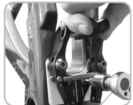
Figure 11.3. Brake attached by two bolts
