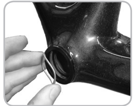
Figure 14.30. Inserting the Wave washer (after the washer) on the non-drive side
