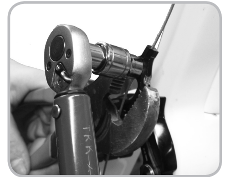
Figure 10.6. Tightening the cable clamp nut
