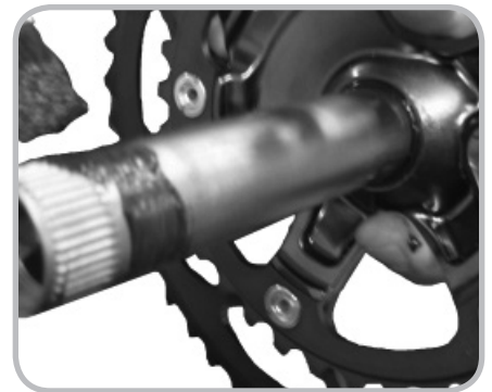
Figure 14.12. Greasing the axle
