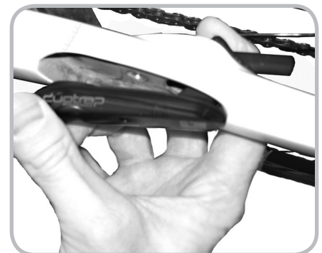
Figure 12.3. Sliding the speed cylinder of a DuoTrap sensor through the chainstay
