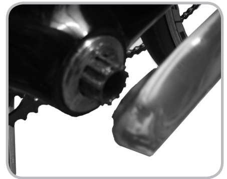
Figure 14.14. Metal bearing cover in place over the bearing
