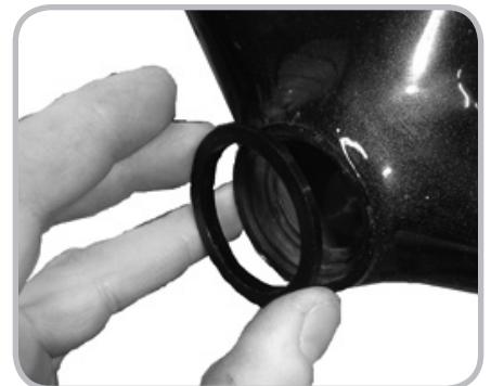
Figure 14.27. Inserting the bearing cups into the bottom bracket shell
