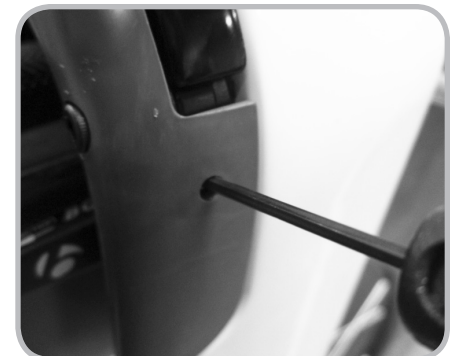
Figure 10.13. Centering screw inside front brake cover
