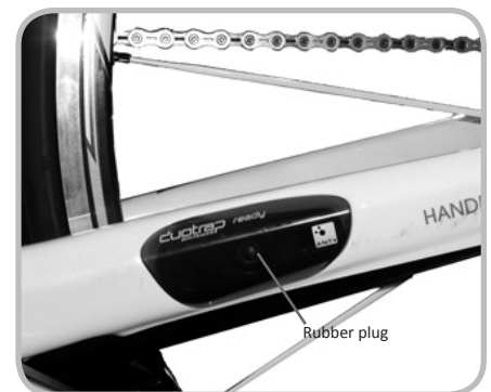
Figure 12.2. Location of attachment bolt
