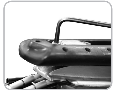
Figure 8.2. Adjusting the tilt and reach of the mono-extension assembly
