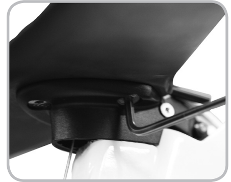
Figure 6.10. Aerobar attachment bolts (three)
