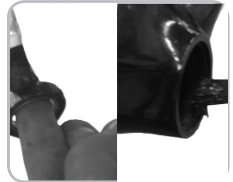
Figure 14.7. Greasing the bearing and the frame saddle
