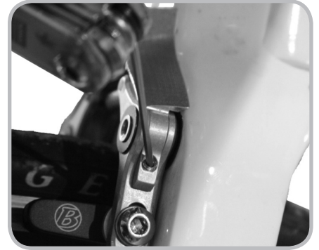
Figure 10.10 Center the brake over the rim
