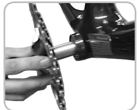
Figure 14.37. Sliding the axle through the bearings
