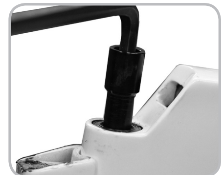
Figure 6.4. Steering axle passes through both bearings, then threads into fork crown
