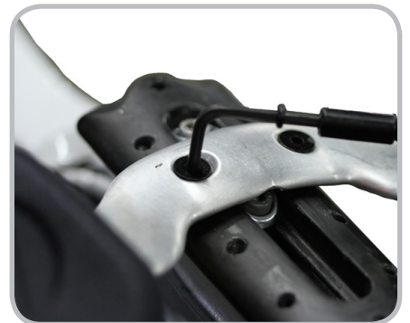
Figure 8.4. Attaching Pad wing to mono-extension
