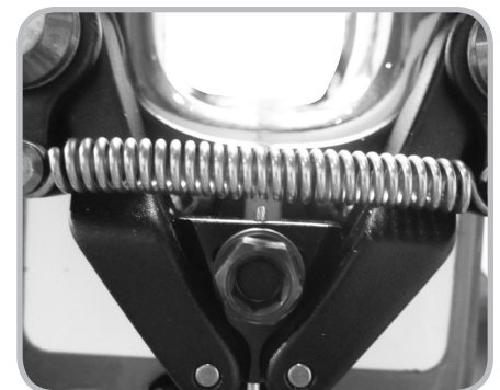
Figure 11.9. Cut cable should not extend past spring.
