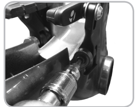
Figure 11.11. Attaching the rear brake cover with two 10 mm bolts
