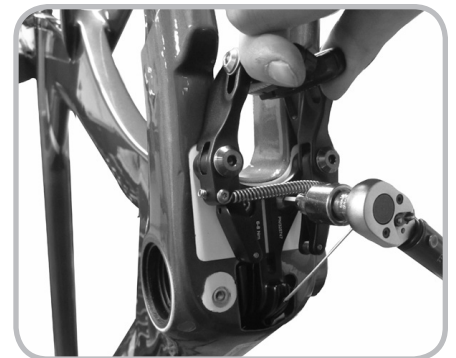
Figure 7.7. Attaching the rear brake
