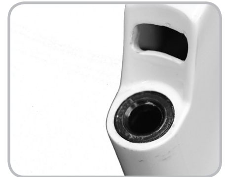
Figure 6.2. Upper head bearing pressed into frame
