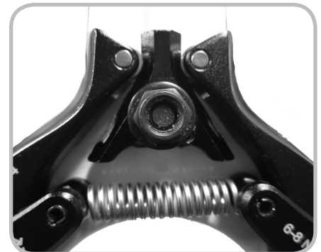
Figure 10.4. Wedge in "home" position between rollers
