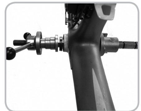
Figure 14.5. Using a headset press to install the bearings
