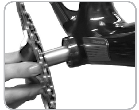
Figure 14.31. Inserting the non-drive side axle
