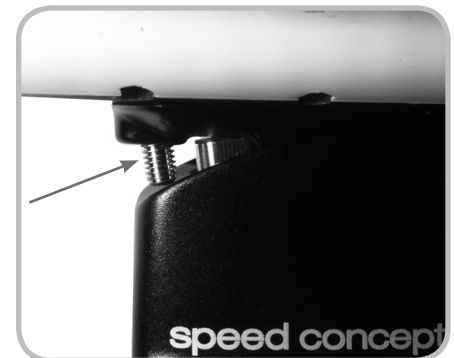
Figure 8.3. Tightening the set screw
