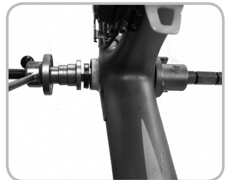
Figure 14.17. Pressing the bearing into the frame
