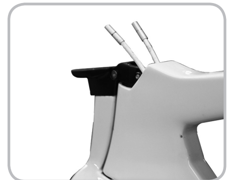
Figure 7.3. Shift housing extending out of the head tube
