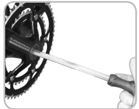
Figure 14.32. Tightening the axle bolt
