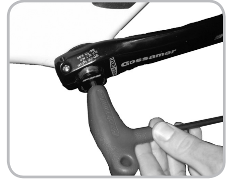
Figure 14.38. Pressing the crank arm onto the axle
