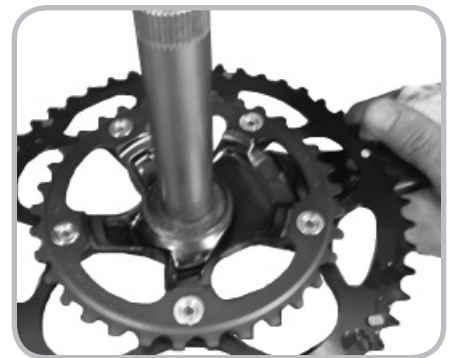
Figure 14.19. Sliding the bearing cover onto the axle
