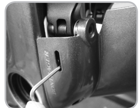
Figure 11.12. Centering the rear brake with cover installed, and without.
