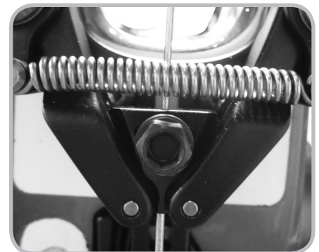
Figure 11.4. Wedge in rollers
