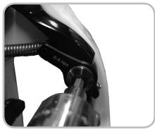
Figure 10.3. Tighten the brake bolts
