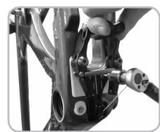
Figure 7.7. Attaching the rear brake
