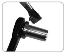
Figure 14.28. Greasing the bearings
