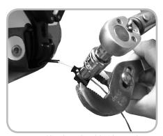
Figure 11.5. Holding the wedge while tightening the cable clamp nut
