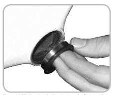
Figure 14.35. Pressing the bearing into the frame with the shield on the outside
