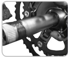
Figure 14.12. Greasing the axle
