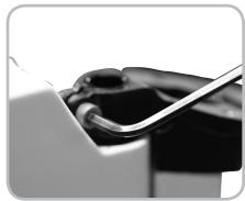
Figure 6.7. Steering axle pinch bolt
