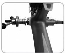
Figure 14.5. Using a headset press to install the bearings
