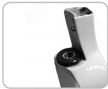
Figure 6.3. Lower head bearing on fork crown
