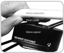
Figure 7.9. Pivot cradle between mono-extension and mono-spacer
