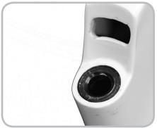
Figure 6.2. Upper head bearing pressed into frame
