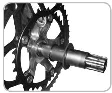
Figure 14.11. Sliding the wave washer and bearing cover onto the axle
