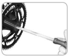
Figure 14.32. Tightening the axle bolt
