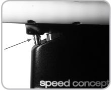
Figure 8.3. Tightening the set screw
