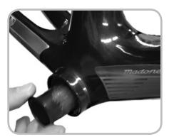
Figure 14.2. Inserting one half of the axle shield into frame
