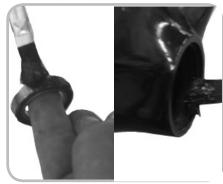
Figure 14.34. Greasing the bearing and the frame saddle
