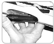
Figure 12.3. Sliding the speed cylinder of a DuoTrap sensor through the chainstay
