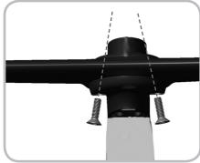
Figure 7.23. Side attachment bolts go in at an angle
