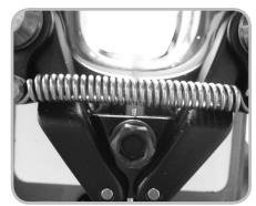
Figure 11.9. Cut cable should not extend past spring.
