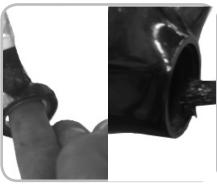
Figure 14.7. Greasing the bearing and the frame saddle
