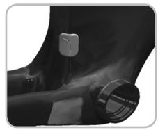
Figure 9.4. Seat tube grommet on cable liner to front derailleur
