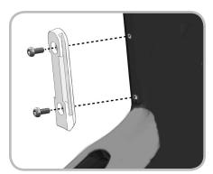
Figure 13.2. Attaching the track to the rear of the seat tube. Note orientation of spring-loaded button.
