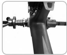
Figure 14.17. Pressing the bearing into the frame
