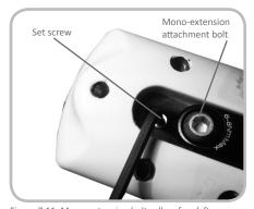
Figure 7.11. Mono-extension bolts allow fore/aft adjustment and control tilt of bar. Set screw prevents movement after adjustment.
