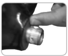
Figure 14.22. Pressing in the second bearing cover
