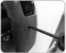
Figure 10.13. Centering screw inside front brake cover
