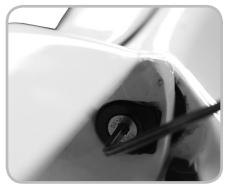
Figure 6.5. Steering lock bolt passes through lock washer and into steering axle
