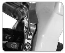
Figure 10.10 Center the brake over the rim
