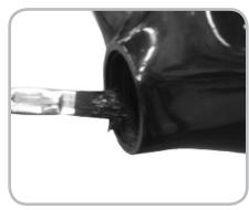
Figure 14.29. Greasing the bearing cups
