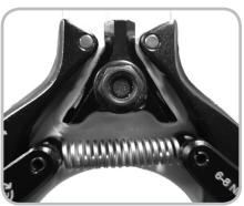
Figure 6.9. Squeeze the lower arms to remove the wedge
