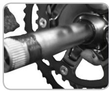
Figure 14.20. Greasing the axle
