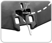
Figure 7.13. T-slot and housing routes through aerobar (bottom view of aerobar)
