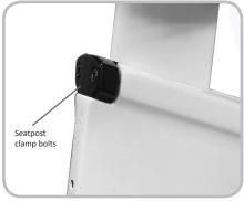
Figure 4.2. Seatpost clamp bolts on the back of the seat tube
