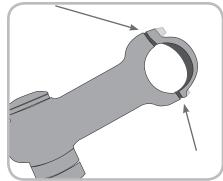
Figure 2.2. Gaps at either end of clamp band
