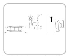
Figure 10.9. Brake pad alignment: carrier aligned with rim, pad face parallel to rim face, slight toe-in
