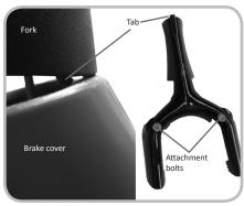
Figure 10.11. Attachment points of front brake cover
