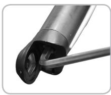
Figure 7.24. Tightening shift lever body
