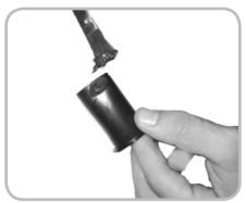
Figure 14.1. Applying grease to the axle shield
