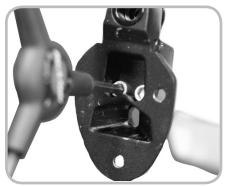
Figure 6.13. Stem attachment bolts (two)
