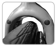
Figure 10.12. Brake cover grommets
