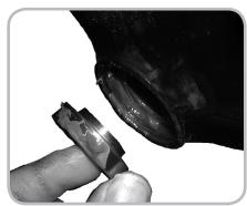
Figure 14.8. Grease on the frame and the non-drive side bearing (with the lip facing in)  $\,$
