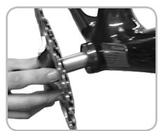
Figure 14.13. Sliding the axle through the bearings
