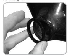
Figure 14.27. Inserting the bearing cups into the bottom bracket shell
