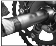
Figure 14.36. Greasing the axle
