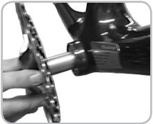
Figure 14.31. Inserting the non-drive side axle
