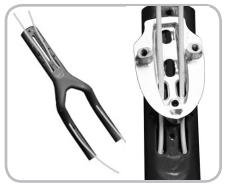
Figure 7.8. Shift housing routed through mono-extension and mono-spacer
