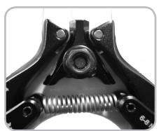
Figure 10.4. Wedge in "home" position between rollers
