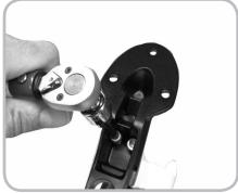
Figure 6.6. Stem-to-fork attachment bolts (two)
