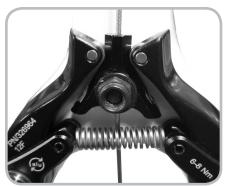
Figure 10.5. Cable in wedge
