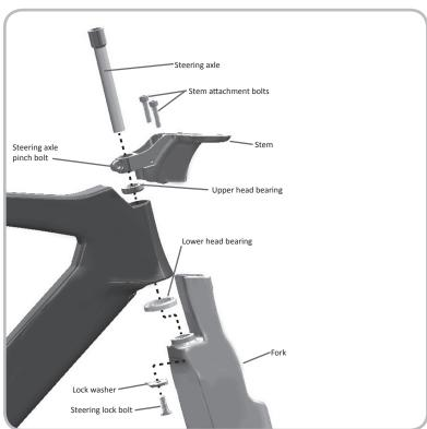
Figure 6.1. Fork attachment exploded diagram
