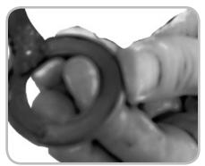
Figure 14.10. Greasing the bearing covers
