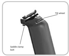
Figure 4.3. Tilt wheel and saddle clamp bolt of saddle angle adjustment mechanism
