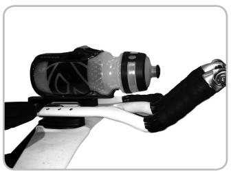
Figure 13.5 Speed Concept bottle cage
