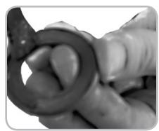
Figure 14.18. Greasing the bearing covers
