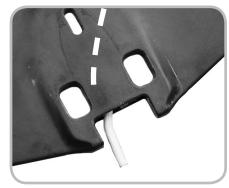
Figure 7.12. Rear brake housing routed out of aerobar (top view of aerobar)
