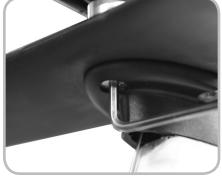
Figure 7.19. Tightening front attachment bolt
