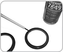
Figure 14.26. Applying LocTite primer to the outer step of the bearing cups
