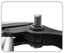
Figure 10.2. E-clip on brake bolt
