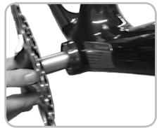
Figure 14.21. Sliding the axle through the bearings
