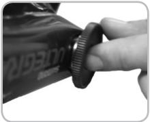
Figure 14.23. Pressing the crank arm onto the axle
