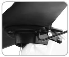
Figure 6.10. Aerobar attachment bolts (three)
