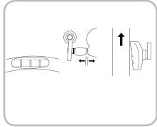
Figure 11.7. Brake pad alignment: carrier aligned with rim, pad face parallel to rim face, slight toe-in
