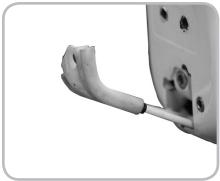
Figure 7.4. Bottom bracket cable guide on shift housing
