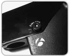
Figure 7.22. Housing cover on stem
