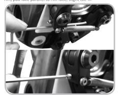
Figure 11.8. Centering the left and right brake pads.
