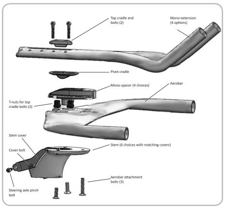
Figure 7.1. Exploded assembly of stem, aerobar, and mono-extension  $% \left( 1\right) =\left( 1\right) \left( 1\right)$
