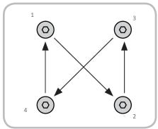
Figure 2.1. Bolt tightening sequence
