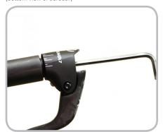
Figure 7.14. Installing brake lever
