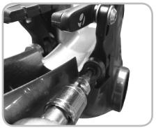
Figure 11.11. Attaching the rear brake cover with two 10 mm bolts  $\,$
