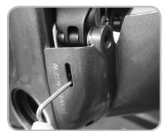
Figure 11.12. Centering the rear brake with cover installed, and without.  $\label{eq:coverage} % \begin{center} \begin{cente$
