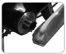
Figure 14.14. Metal bearing cover in place over the bearing
