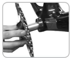
Figure 14.37. Sliding the axle through the bearings
