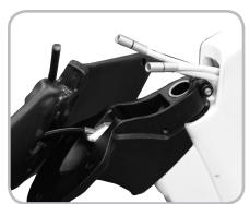
Figure 7.18. Installing the aerobar, ferrule in long position
