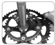
Figure 14.19. Sliding the bearing cover onto the axle
