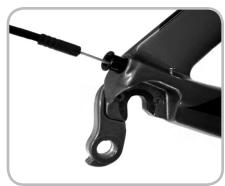
Figure 9.5. Rear derailleur cable passing through the dropout housing stop
