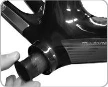
Figure 14.41. Inserting one half of the axle shield into frame
