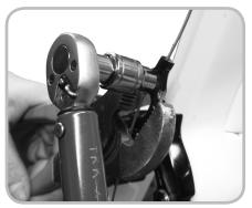
Figure 10.6. Tightening the cable clamp nut
