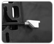
Figure 7.15. Front brake ferrule
