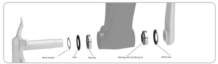
Figure 14.6. SRAM bearing set
