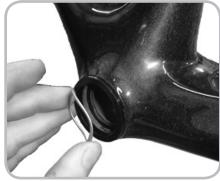
Figure 14.30. Inserting the Wave washer (after the washer) on the non-drive side
