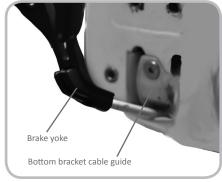
Figure 7.6. Brake yoke with housing connected
