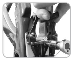
Figure 11.3. Brake attached by two bolts
