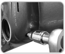
Figure 11.10. Attaching the rear brake cover with front 20 mm bolt
