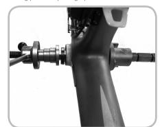
Figure 14.9. Pressing the bearing into the frame
